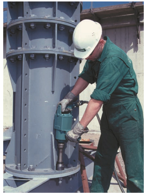
3/4" Drive Hydraulic Impact Wrench
