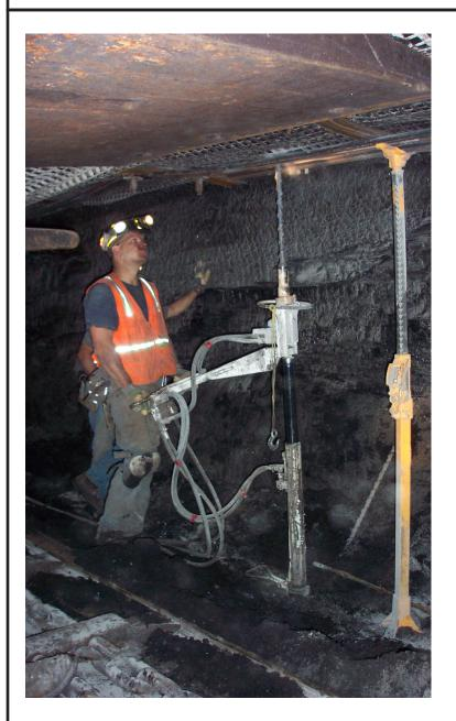
A well-balanced, portable, hydraulic roofbolter prefect for underground drilling and bolting operations. Made in the USA by MPI Supply.
