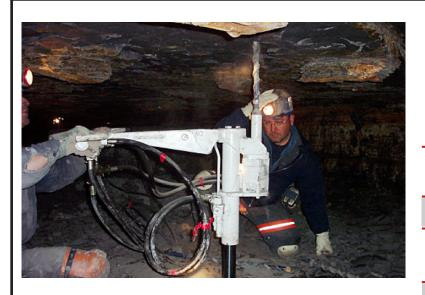
Low profile, portable handheld hydraulic roofbolter. Made in the USA by MPI
